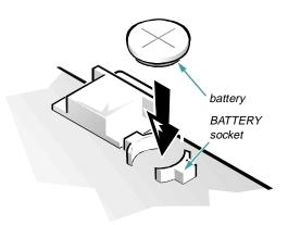
Figure 6-14. System Battery and Battery Socket
