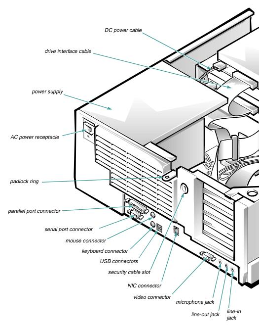
Figure 5-6. Inside the Chassis
