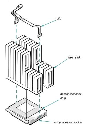
Figure 6-13. Installing the Heat Sink
