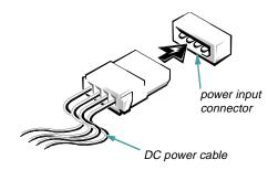
Figure 7-4. DC Power Cable Connector
