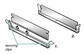
Figure 6-7. Installing a DIMM
