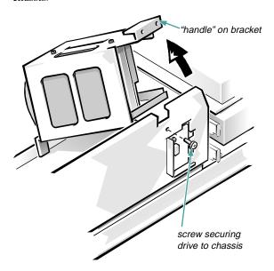
Figure 7-10. Removing the Hard-Disk Drive Bracket
