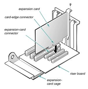
Figure 6-5. Installing an Expansion Card
