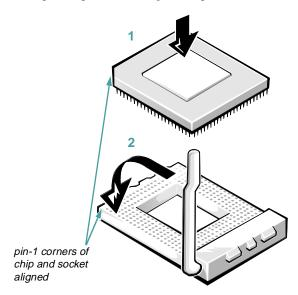
Figure 6-12. Installing the Microprocessor Chip
