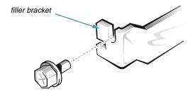
Figure 6-4. Removing the Filler Bracket
