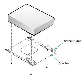
Figure 7-7. Attaching the New Bracket to the New Drive
