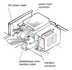
Figure 7-9. Attaching Diskette Drive or Tape Drive Cables
