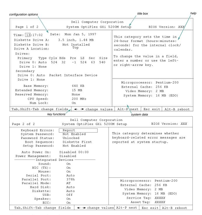
Figure 2-1. System Setup Screens
