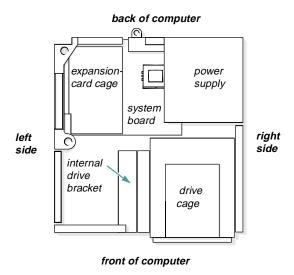
Figure 5-5. Computer Orientation View
