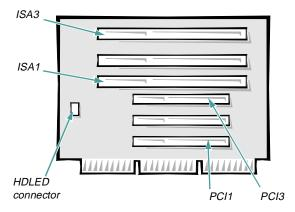
Figure 6-3. Riser-Board Expansion-Card Connectors
