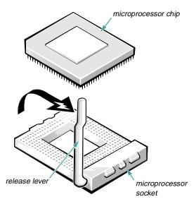
Figure 6-10. Removing the Microprocessor
