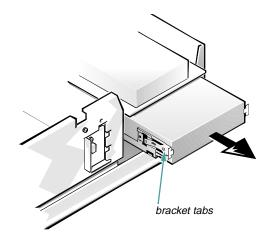
Figure 7-6. Removing a Drive
