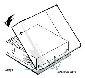
Figure 5-4. Replacing the Computer Cover
