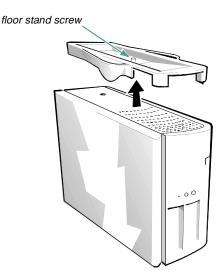
Figure 5-2. Removing the Floor Stand
