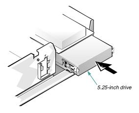
Figure 7-8. Inserting the New Drive Into the Drive Bay
