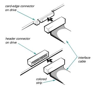
Figure 7-5. Drive Interface Connectors
