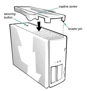
Figure 1-1. Attaching the Floor Stand
