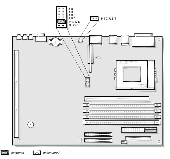
Figure 5-7. System Board Jumpers
