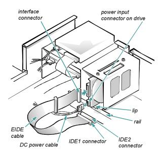
Figure 7-12. Attaching Hard-Disk Drive Cables
