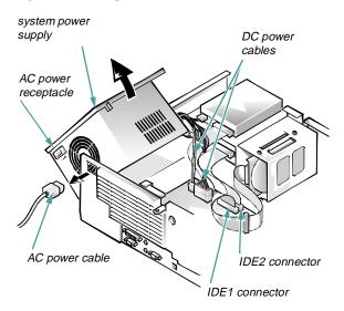
Figure 5-9. Rotating the Power Supply
