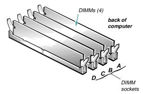
Figure 6-6. DIMMs and DIMM Sockets
