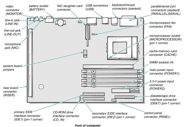
Figure 6-1. System Board Features
