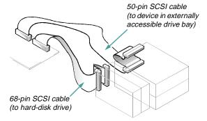
Figure 7-13. Internal SCSI Cable
