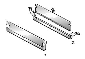
Figure 6-8. Removing a DIMM
