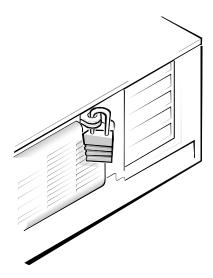
Figure 5-1. Padlock Installed
