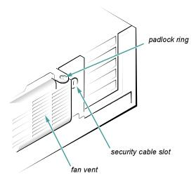
Figure 1-2. Security Cable Slot
