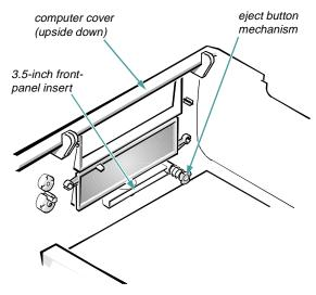
Figure 7-3. Removing the Front-Panel Insert for the 3.5-Inch Bay
