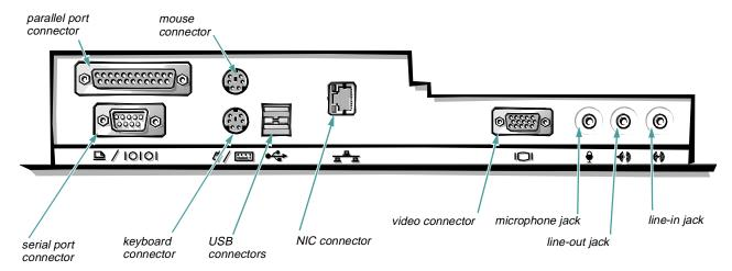
Figure 4-1. I/O Ports and Connectors
