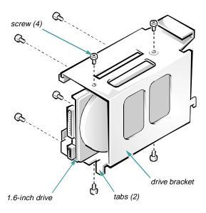
Figure 7-11. Inserting the Hard-Disk Drive in the Bracket
