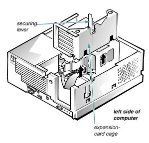
Figure 5-8. Removing the Expansion-Card Cage
